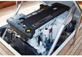
struts. (The engine air intakes are clandestinely placed beneath the gunwales.) With the box elevated, I had plenty of room to check both oil and coolant; the duplex Racors and seawater strainer were not as accessible. The Racors were below deck level and faced inboard, so it would be a bit
