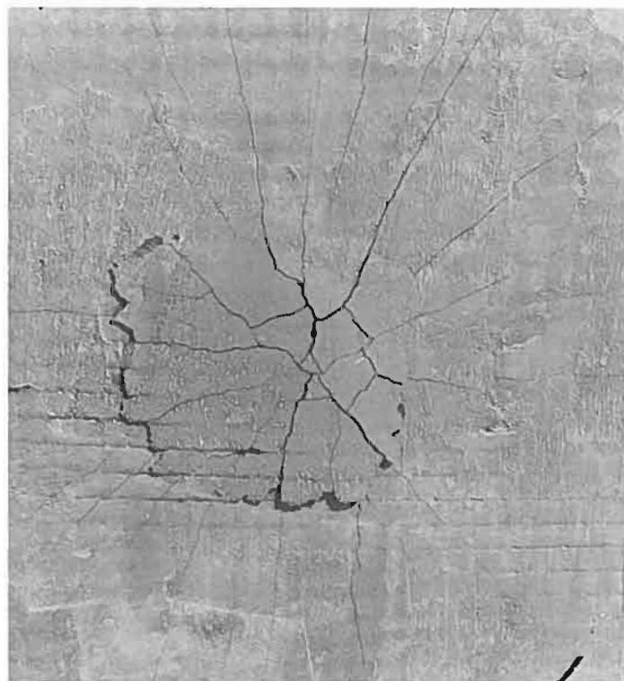
Fig. 9 (a) and (b). Bottom side of panel 55 after drop-impact test. (3 + 2 layers 1/2-ga. hardware cloth, deformed double-drawn rods at 4 in.) (Compare with Fig. 5)
