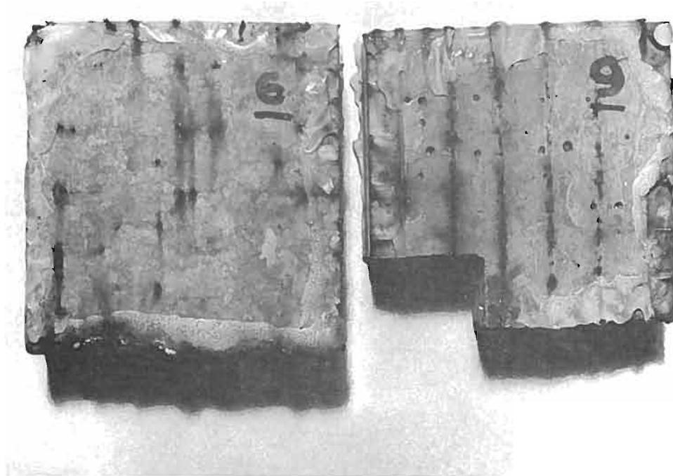
Fig. 32. Rust staining on bottom surface of coupons containing (a) 1/2-22 ga. hexagonal mesh with light zinc coating and (b) 1/2-ga. welded square mesh with zinc coating removed.
