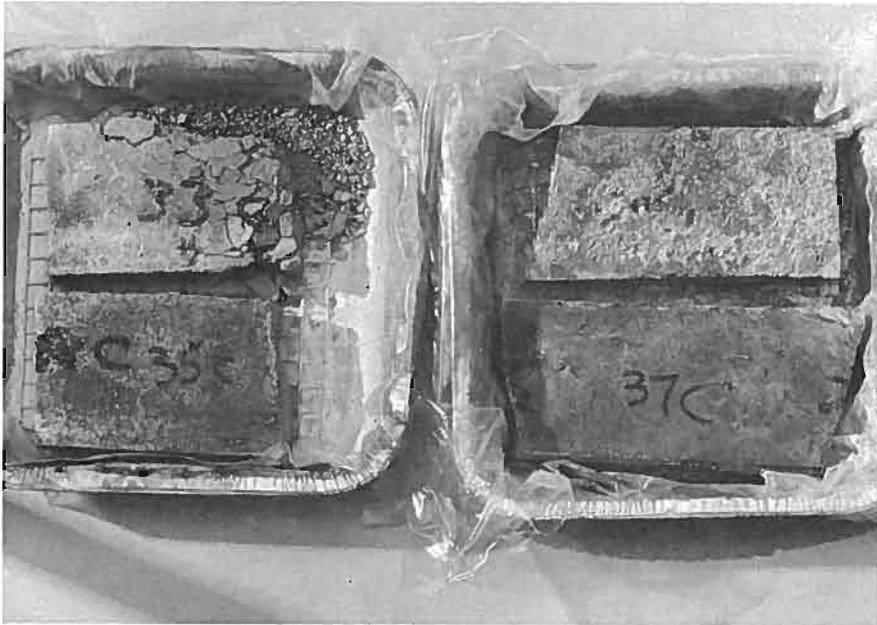
Fig. 28. Breakdown of unreinforced coupons after 350 freeze-thaw cycles.
