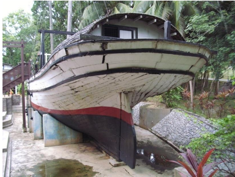
Photo 4.45. Cargo carrier 'Kemajuan T.65' built in 1946, 34.5 m long, 10.4 m beam, 4 m draft. Terengganu State Museum, Kuala Terengganu.
