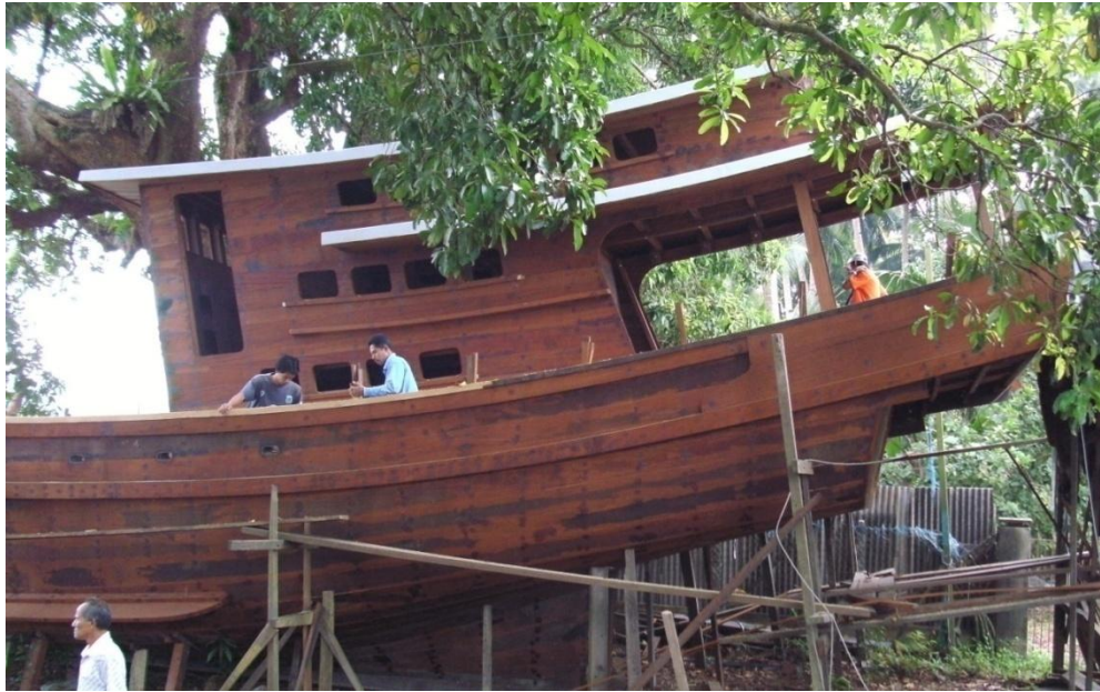
Photo 5.2. Overhung transom and underwater design with new construction of Class B fishing boat. Kuala Terengganu.
