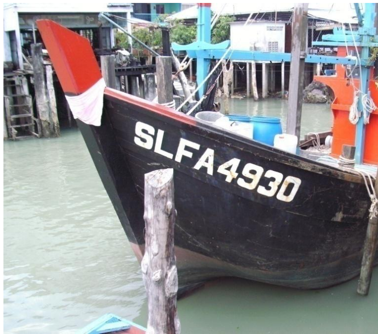
Photo 4.11. Unusual bow design creating large holding capacity with no GRT penalty. Note also the large stem post. Pulau Ketam.
