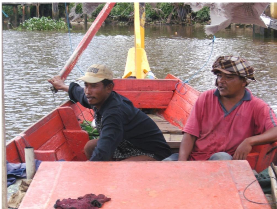
Photo 4.57. Uplifted tiller goes over stern post. Kota Bharu.
