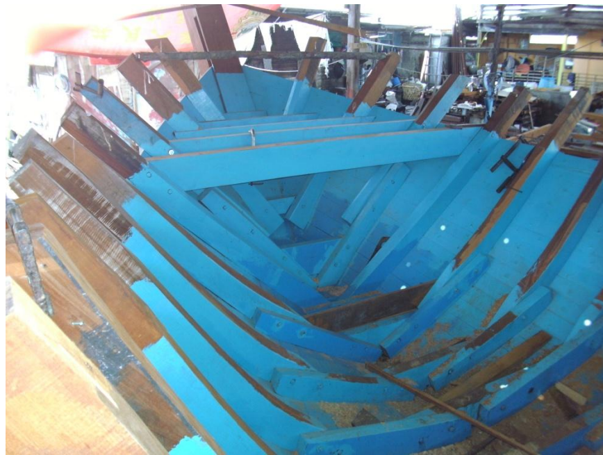
Photo 4.14. V shaped cross section towards bow at PK1 boatyard. Pulau Ketam.
