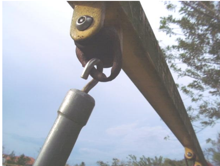
Photo 4.40. Heavily worn linkage for child's swing at public playground. Skudai.
