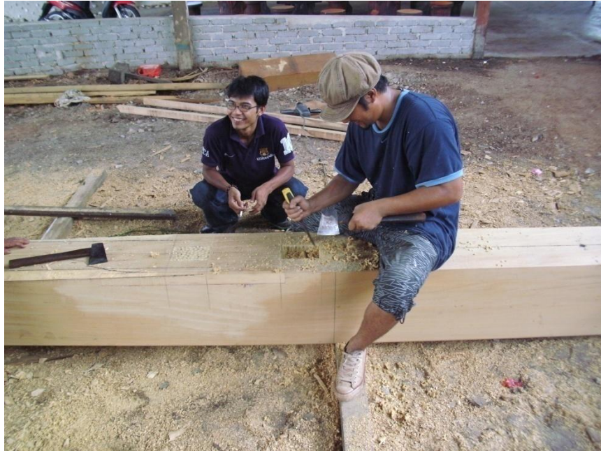
Photo 5.5. Penetrations into keel bar, sharp corners produce high stress concentrations. Kuala Terengganu.
