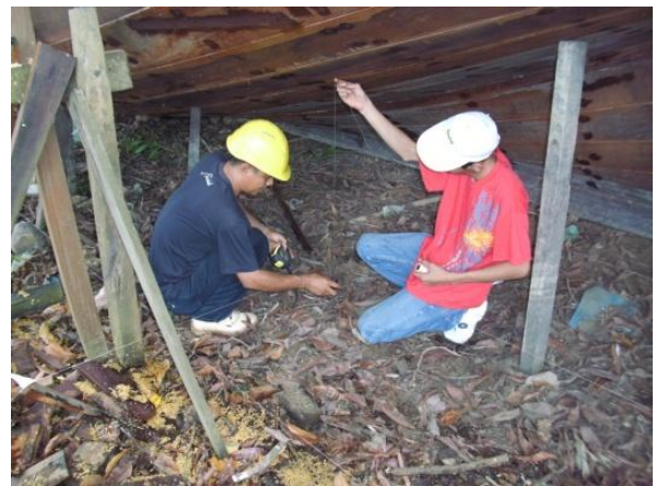
Photo 3.4. Measuring verticals from grid
