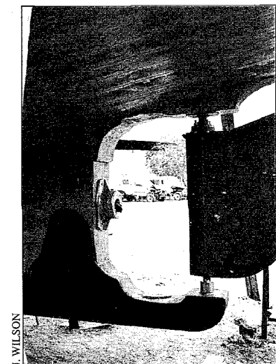
Photo 2 Filling the propeller aperture with fashion pieces, particularly forward of the propeller, reduces efficiency and increases vibration
