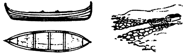
Fig. 727. Surf-landing boat as used in Northern Norway where there is upwelling surf. Boat is 20×5×2 ft. (6.1×1.52×0.6 m.)
