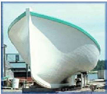
Northumberland Strait Boat The shadows clearly highlight the flare on this new, yet-unnamed Northumberland Strait boat. The narrow wood planks can also be detected. (Courtesy: David Walker)
