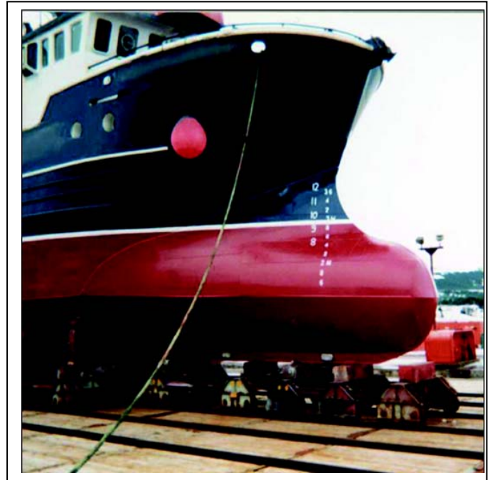
Figure 13: F/V "Royal Mariner" after having bulbous bow fitted
