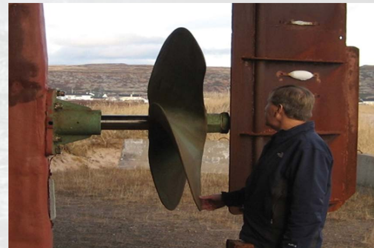
Proper Sizing of Propeller and selection of RPM; Bigger slower propeller is more efficient
