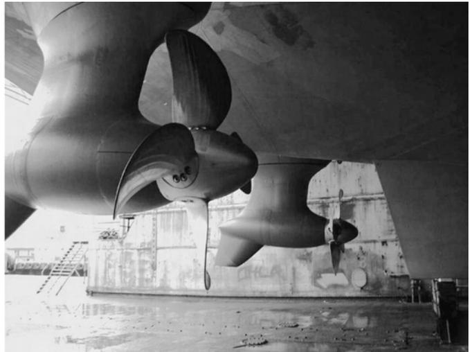
Figure 2.49. Azimuth thrusters by Rolls-Royce that can operate up to 24 knots. The figure on the left illustrates the Z-drive. The right picture shows the two thrusters working as tractor propellers.
