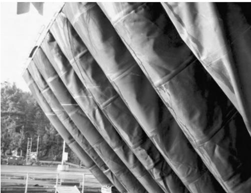
Figure 5.2. Details of the bow seal (skirt) of an SES. (Photo: Hans Olav Midtun.)
