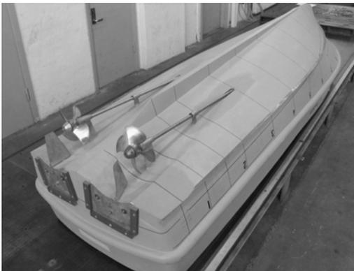
Figure 2.2. Propellers with inclined shafts installed on a model of a planing vessel with hard chines. Propeller tunnels are used to minimize the shaft angle. The rudders are twisted and adapted to the propeller slip stream. Two interceptors are placed at the transom to control the trim angle (see section 7.1.3 and Figure 7.5 for more details about interceptors). (Photo by K.A. Hegstad)
