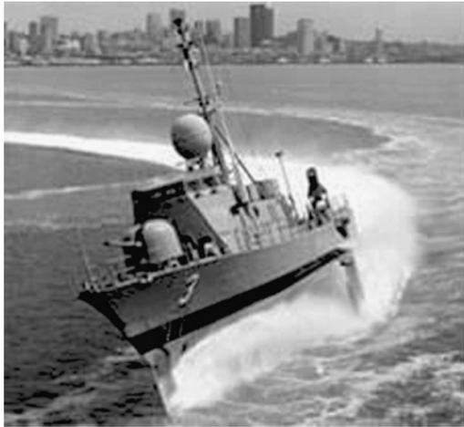
Figure 6.20. The PHM hydrofoil vessel by Boeing (Johnston 1985).
