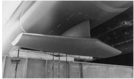
Figure 7.3. T-foil placed below the keel and used to damp vertical wave-induced ship motions at high speed (Seastate).
