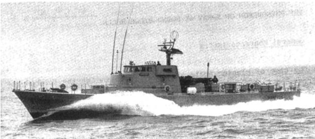
Figure 2.22. Development of spray at a semi-displacement round-bilge hull (Müller-Graf 1991).
