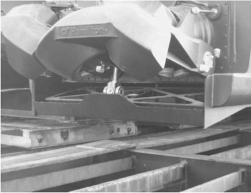
Figure 7.4. Trim tab installation (Seastate). The trim tab is an elongation of the hull bottom. By changing the angle of the trim tab by means of an hydraulic actuator, the trim moment on the ship is changed so that the trim angle is either increased or reduced.
