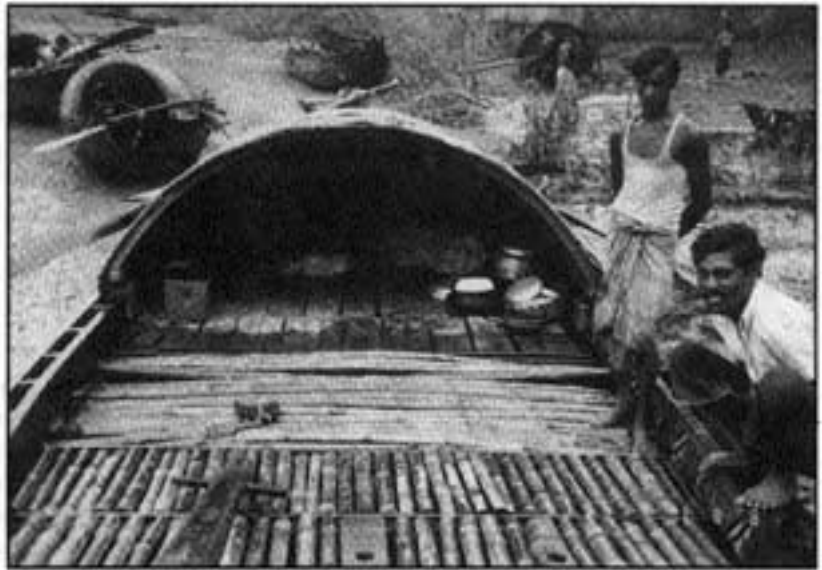
The split bamboo deck and cooking utensils aboard a chandi boat.
