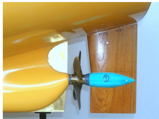
Figure 16 – Bulk carrier ship model with rudder bulb
