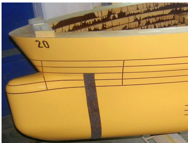
Figure 17 – Proposed fore body modification for a Tanker conversion project
