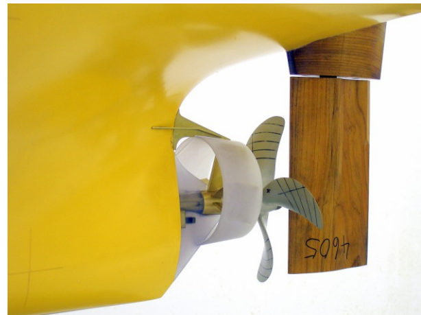
Figure 12 – Bulk carrier model with BMS Mewis Duct®
