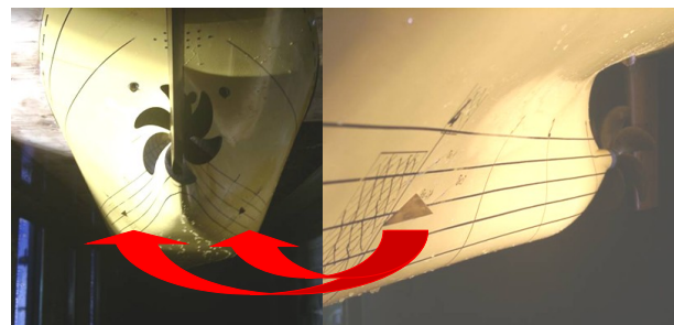
Figure 10 – Arrangement of VG-fins at a Container Vessel
