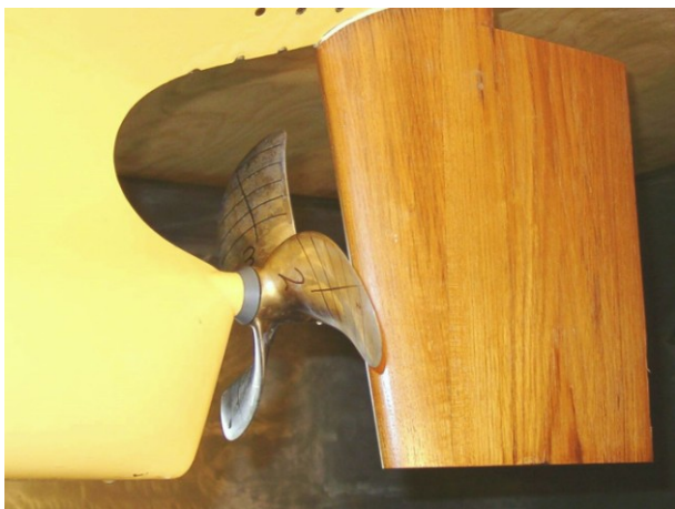
Figure 13 – VLCC ship model tested with a 3-bladed propeller designed by MMG
