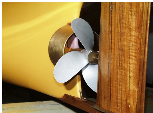
Figure 11 – Sumitomo Integrated Lammeren Duct (SILD)
