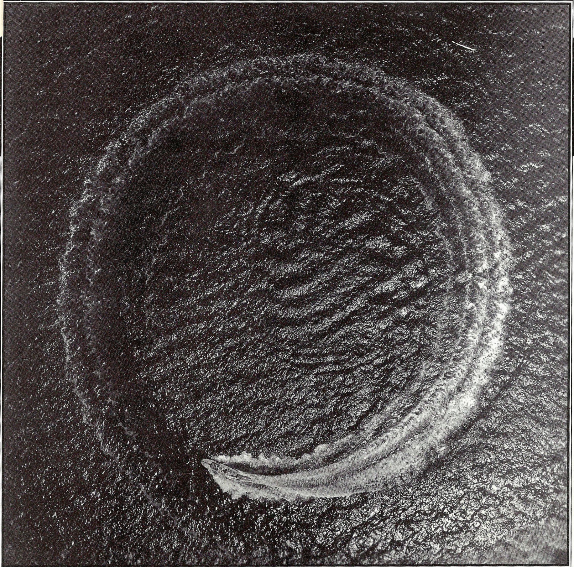
A 63' aircraft rescue boat carves a starboard turn at full speed, full rudder, within a turning diameter of 646'. The author's many years of engineering high-speed military craft such as this—and then systematically studying their performance—led to the design “rules of thumb” for twin-screw rudders on the following pages.
