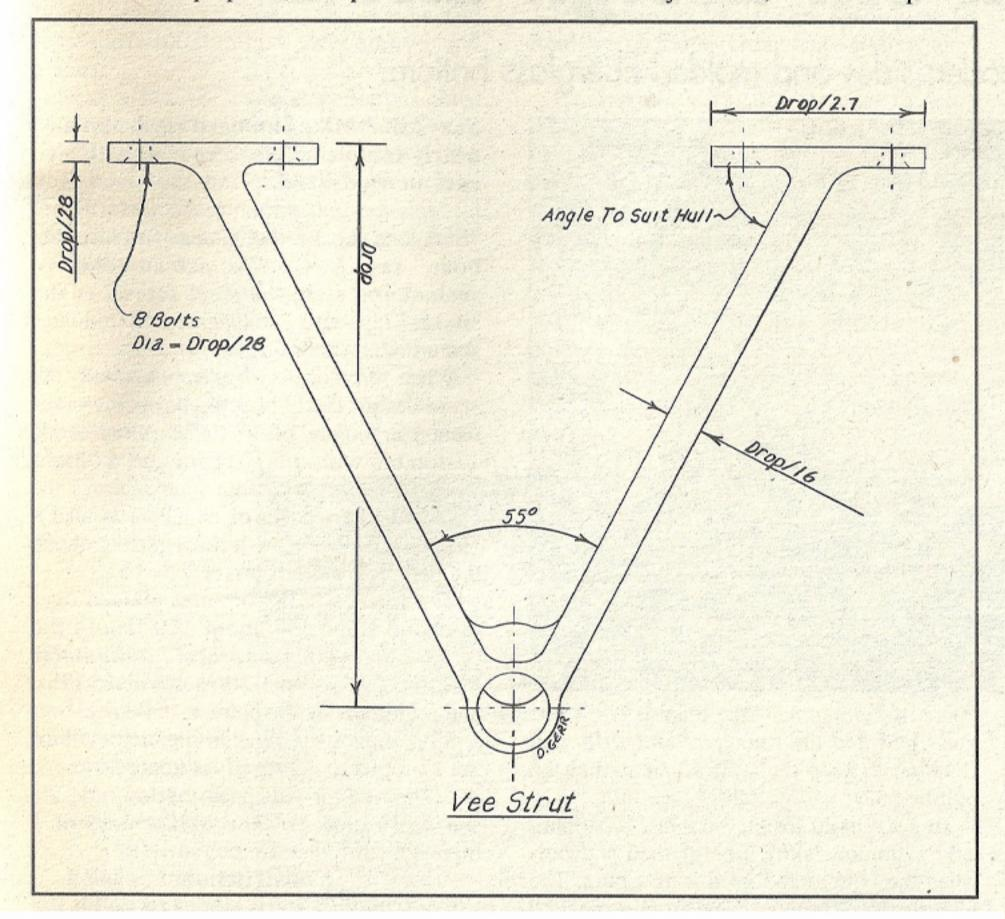
it is to concentrate on obtaining unobstructed flow to the propeller. Perhaps the vessels that most frequently run into problems here are traditional down-east Maine lobster boats that have been powered to run at 20 knots and faster.
