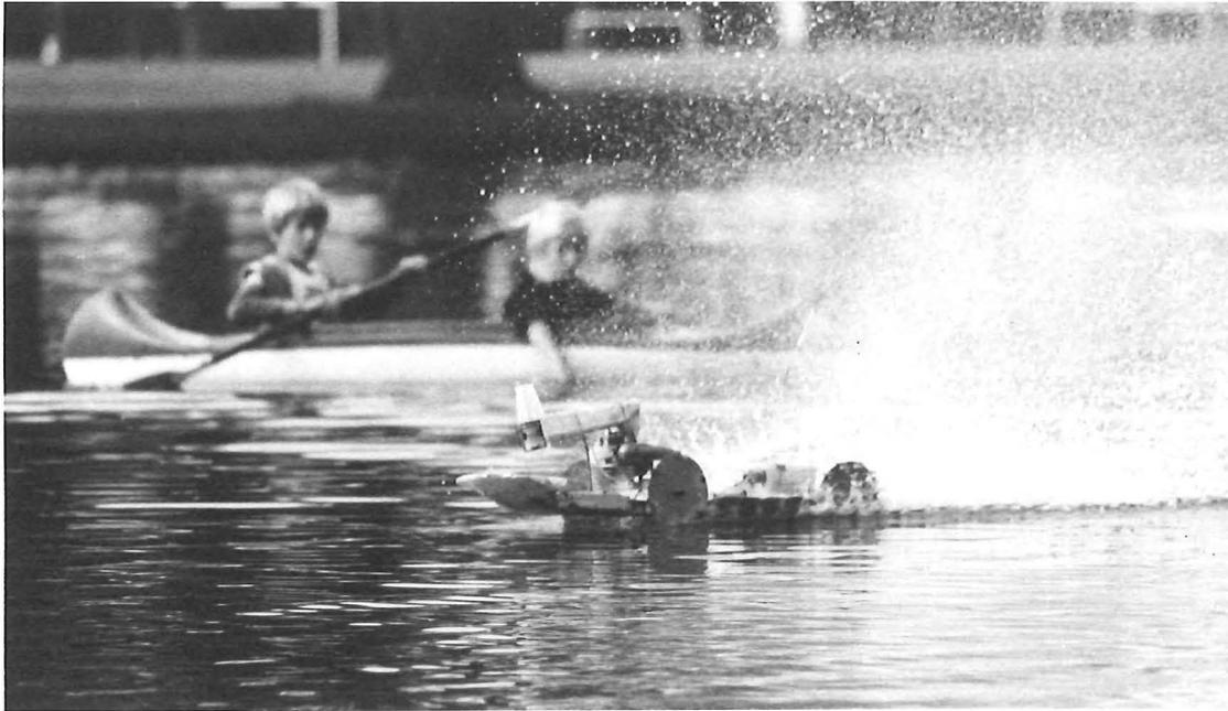
FIGURE 12·12: THE MODEL IN THE PLANING-PLANING CONDITION. THE REAR OF THE HULL IS IN THE WATER, AND THE REAR WHEELS DEEPLY IMMERSSED ( $d/D \doteq 0.3$ ,  $V_0 \doteq 4\text{m/s}$ , WHEELS: F 8, R 20)
