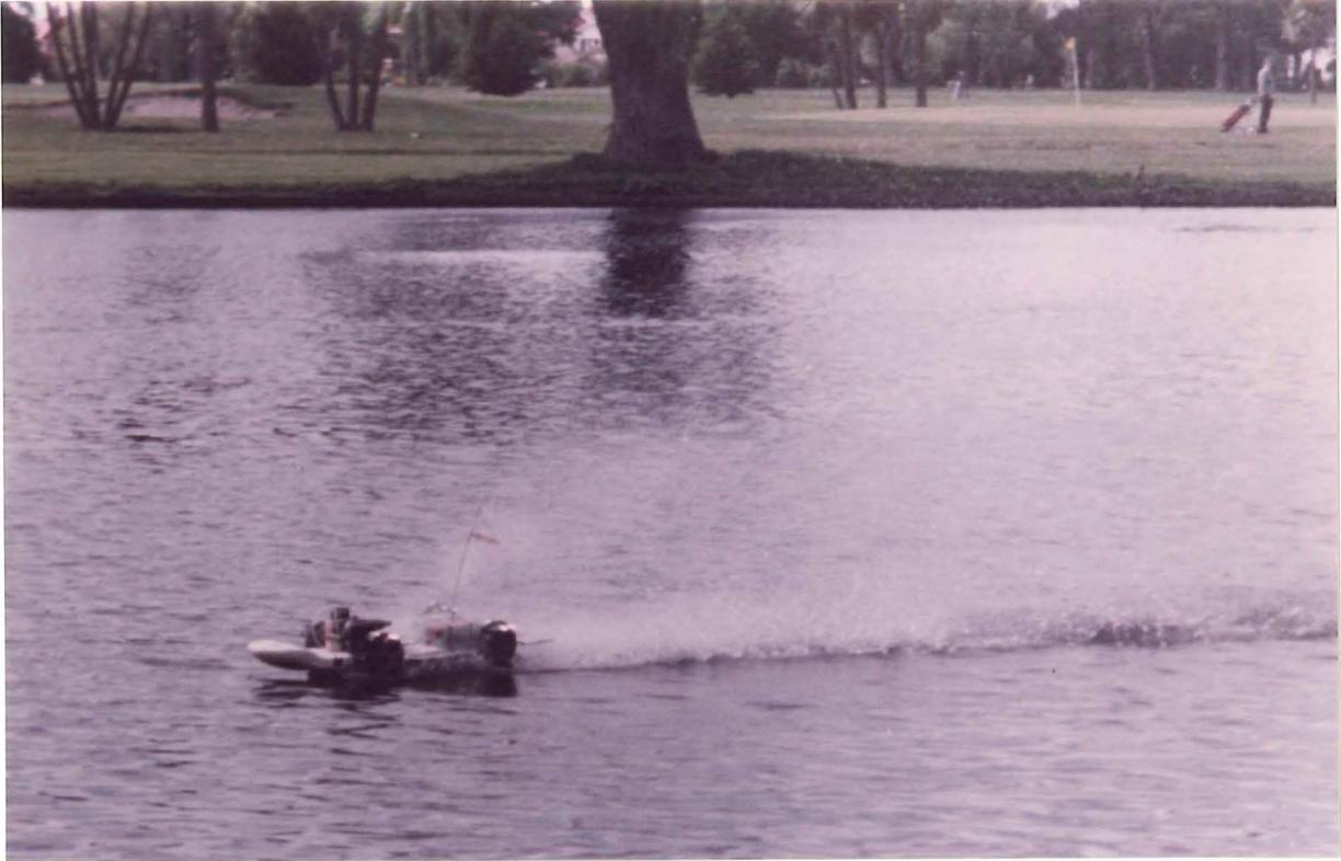
FIGURE 12.20: THE SHORT WHEELBASE MODEL WITH BEST WHEEL DESIGN (WHEEL NO.17) IN THE PLANING-FLYING CONDITION AT ABOUT 9 m/s. NOTE THE VERY SMALL IMMERSION AND ONLY A LITTLE SPRAY; NO AIR CLEANER WAS REQUIRED AT SPEED.
