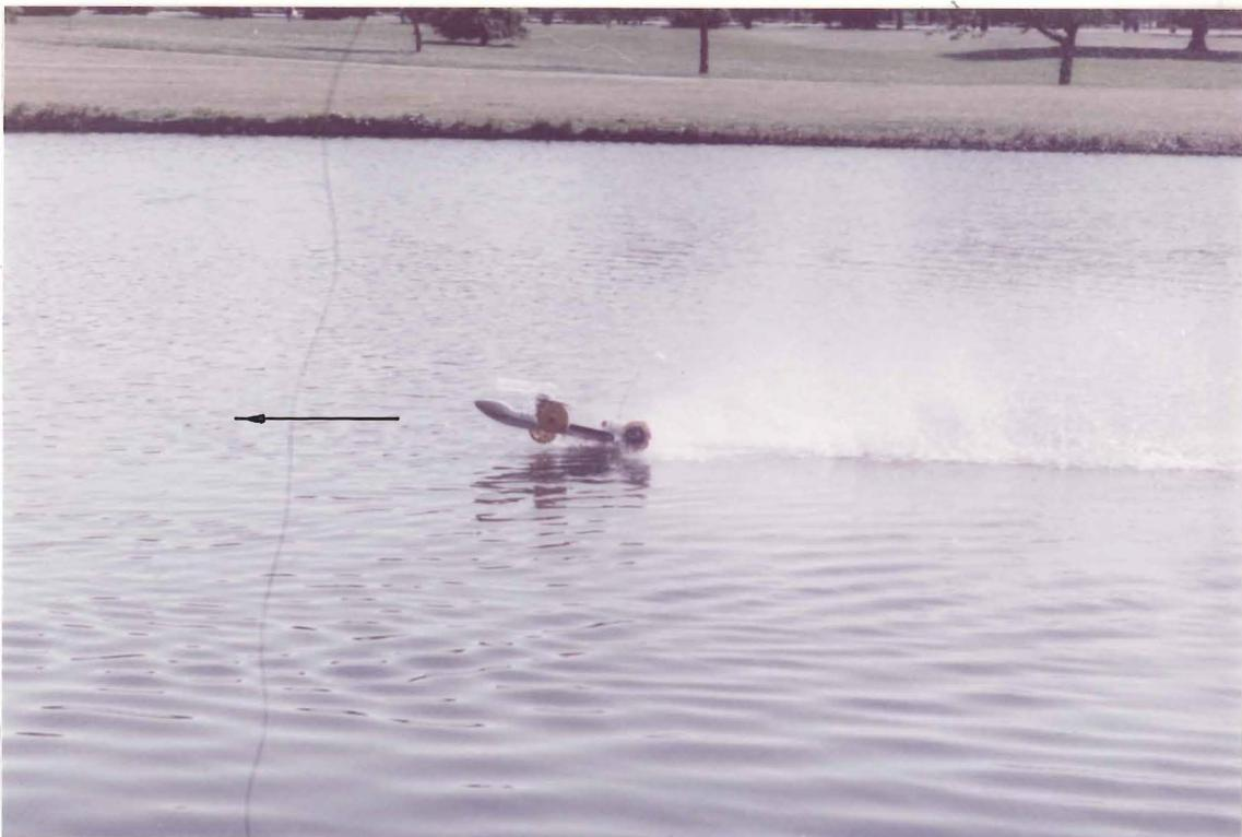
FIGURE 12.19: WHEN THE BOUNCING WAS EXCESSIVE THE MODEL LEFT THE WATER COMPLETELY. STEERING WAS DIFFICULT UNDER THESE CONDITIONS. (WHEELS F7, R19)
