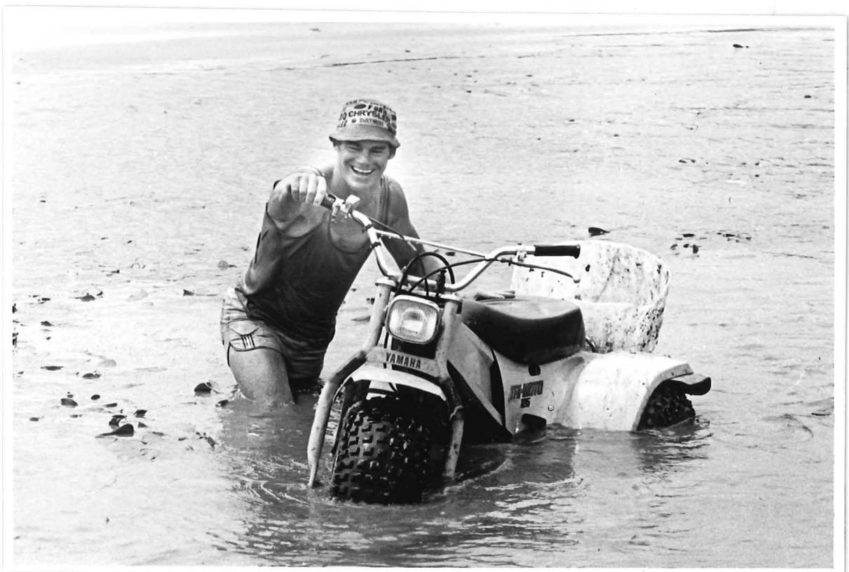
FIGURE 2-14: YAMAHA 125 BALLOON TYRED AMPHIBIOUS THREE WHEELER. (Auckland Star photos)
