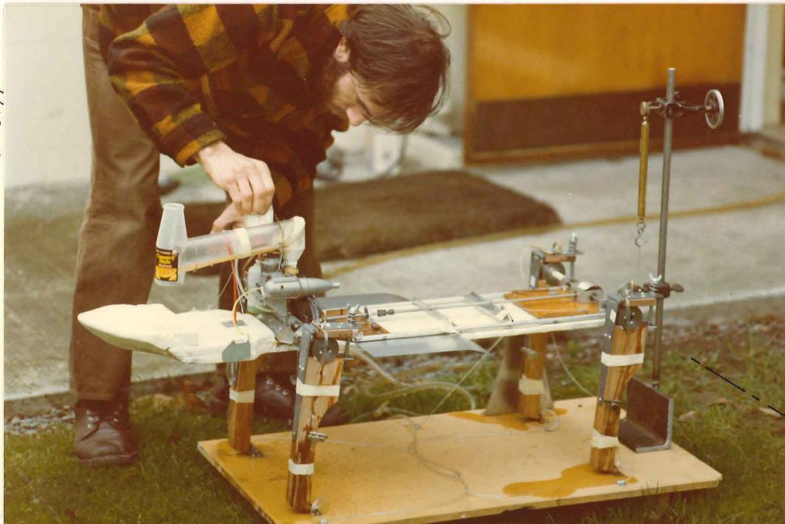
FIGURE 12.10: THE DYNAMOMETER IN PREPARATION FOR TESTS WITH THE LONG WHEELBASE VERSION OF THE MODEL
