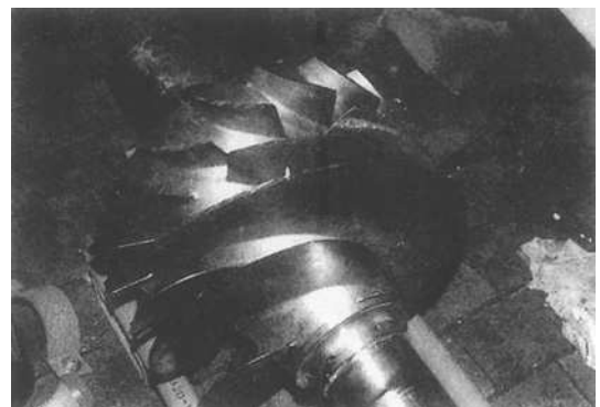
Figure 16.4 Typical inducer design
