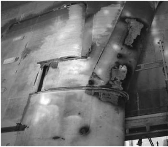
Figure 9.39 Example of rudder erosion
