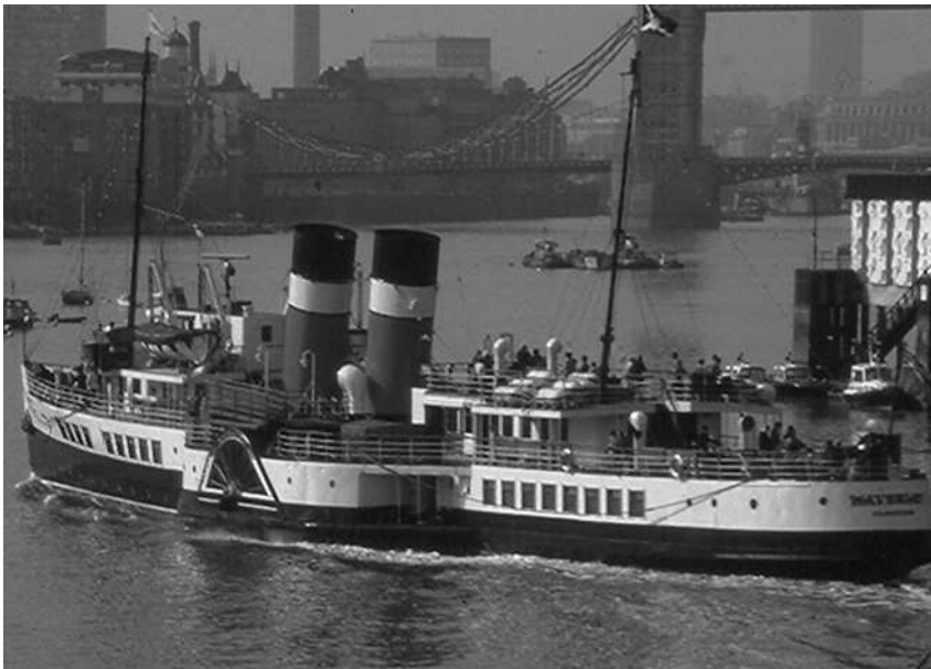
Figure 2.14 P.S. Waverley : Example of a side wheel paddle steamer
