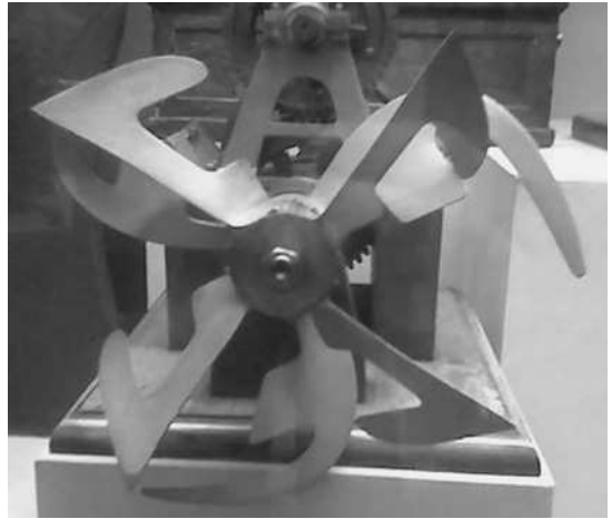
Figure 1.11 de Bay's contra-rotating propeller design
