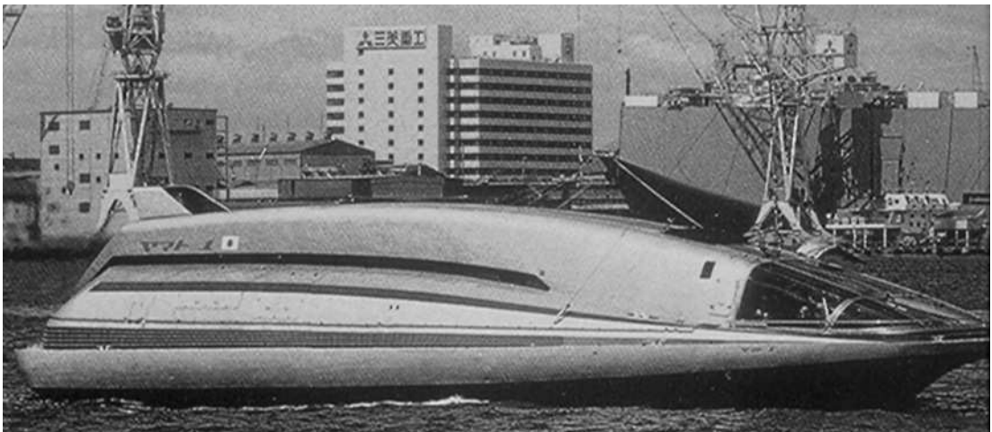
Figure 2.19 Yamato 1 : Experimental magnetohydrodynamic propulsion craft
