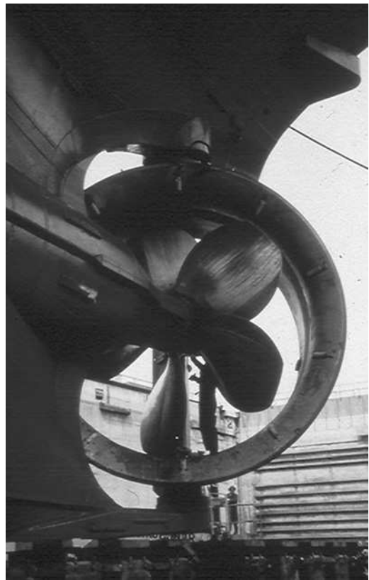
Figure 2.5 Steerable ducted propeller
