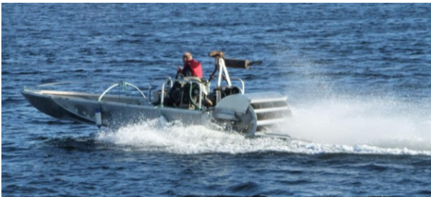
Figure 7: Cupped float wake fountain
