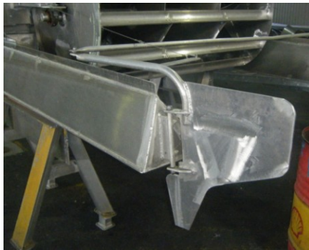
Figure 2: Hull extensions and rudder modifications
