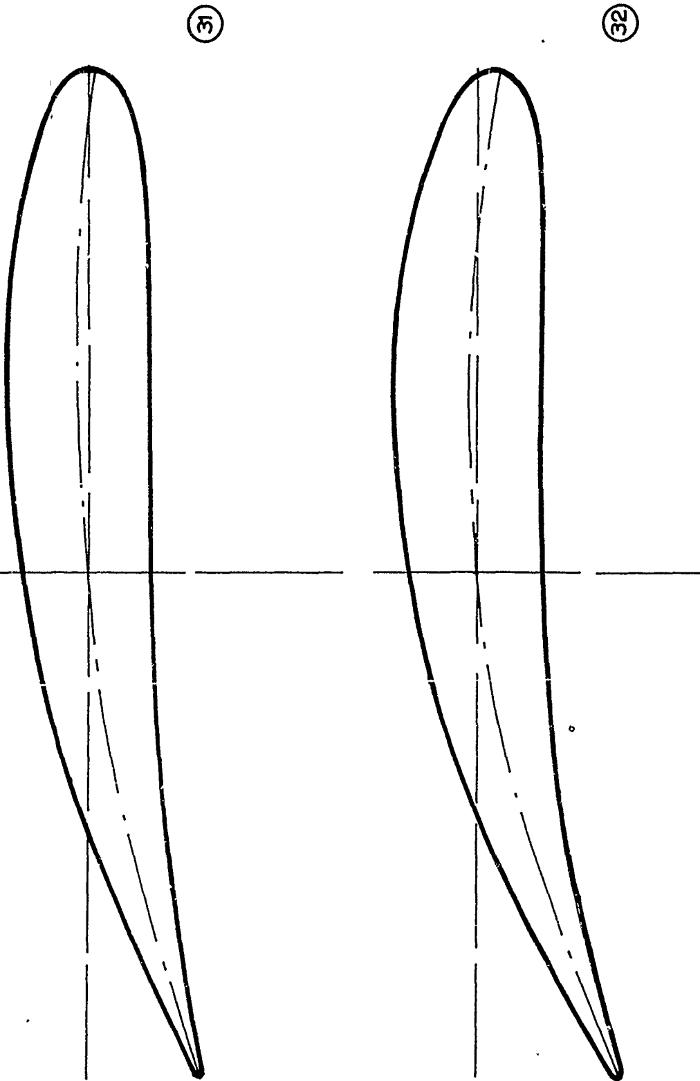
Figure 13. Camber and thickness distribution of nozzles selected for experiments
