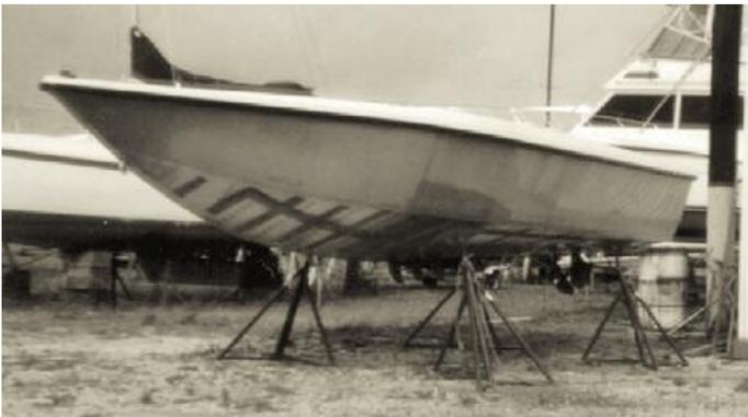
Figure 32 Recreational ski boat from Hydrodyne. Translucent hull makes location of manometer taps visible in this view. Figure reproduced from Royce (2001).
