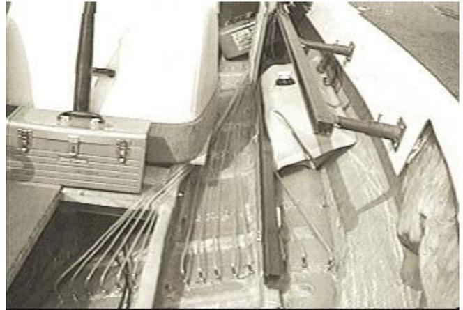
Figure 33 Row of manometer taps in hull of Hydrodyne ski boat. Figure reproduced from Royce (2001).
