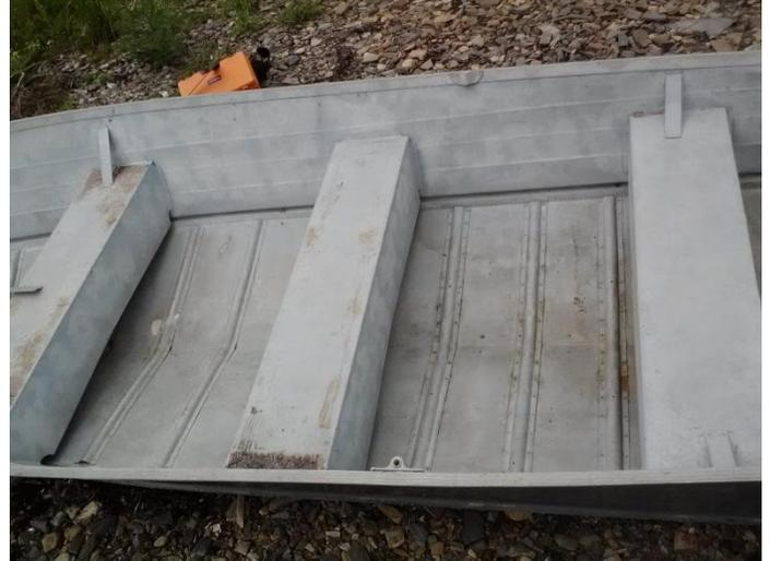
Figure 6 Structure of aluminum fishing boat. Transverse stiffeners are visible on the hull.
