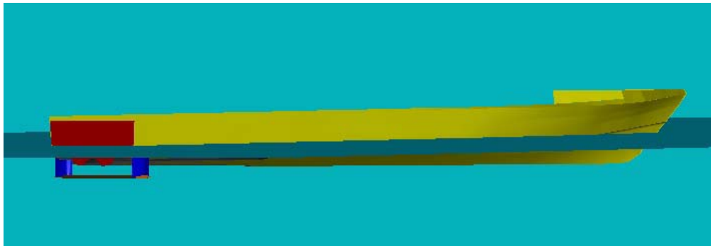
Figure 5.5 : The High Speed Craft (M Hull) incorporated with Stern Foil
