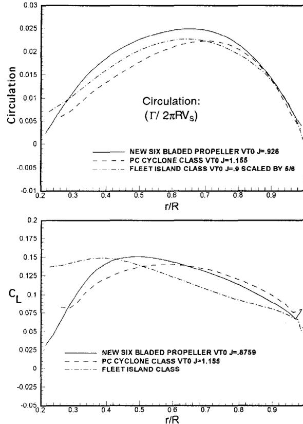
Fig. 15. Comparison of circulation and lift coefficient between *ISLAND* Class and *CYCLONE* Class propellers
