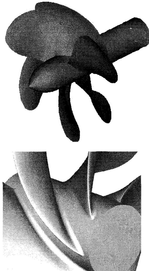
Fig. 21. Computer renderings of *ISLAND* Class 6-bladed propeller
