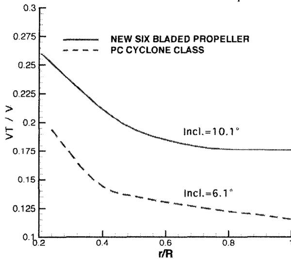
Fig. 14. Comparison of tangential velocities between *ISLAND* Class and *CYCLONE* Class
