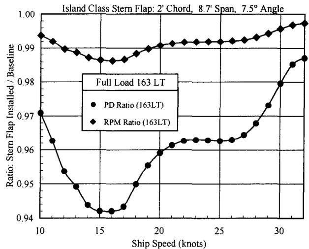
Fig. 8. Projected full-scale stern flap performance on *ISLAND* Class, full load condition of 163.39 tons
