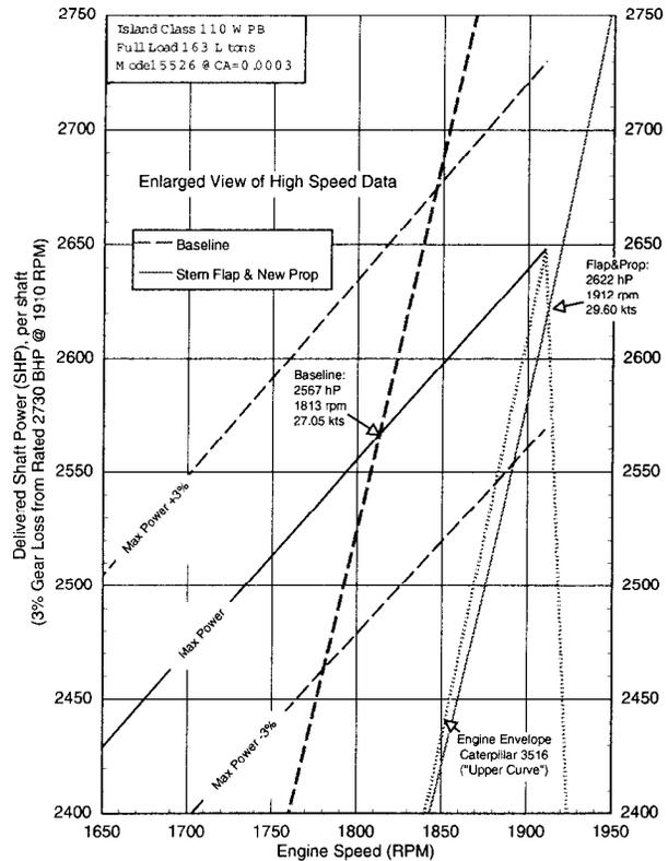
**Fig. 23.** ISLAND Class main engine operating envelope (Caterpillar 3516), with projected shaft powers baseline vs. stern flap and new 6-bladed propeller, full load condition
