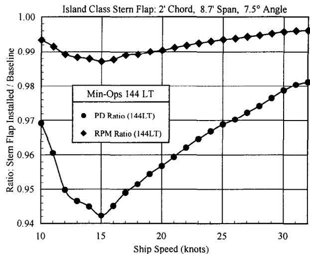
Fig. 9. Projected full-scale stern flap performance on *ISLAND* Class, min-ops condition of 143.6 tons
