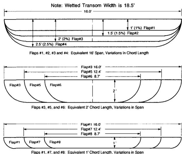
**Fig. 3.** Sketch of model-scale stern flaps
