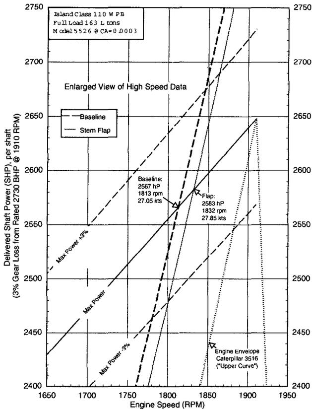
**Fig. 10.** ISLAND Class main engine operating envelope (Caterpillar 3516), with projected shaft powers baseline vs. stern flap, full load
