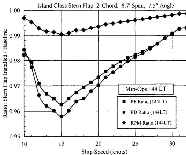
Fig. 6. Model-scale performance of selected stern flap #6, Min-Ops condition of 143.61 L. tons
