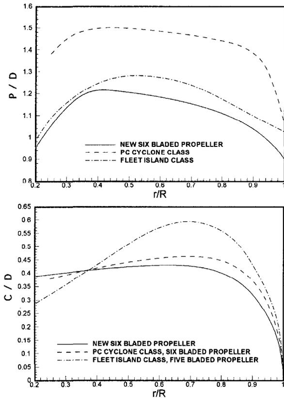
Fig. 19. Propeller geometry parameters, pitch and chord
