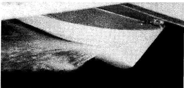
**Fig. 12.** Model-scale bow spray comparison, baseline (upper) and with bow spray rails installed (lower), full load, 28 knots
