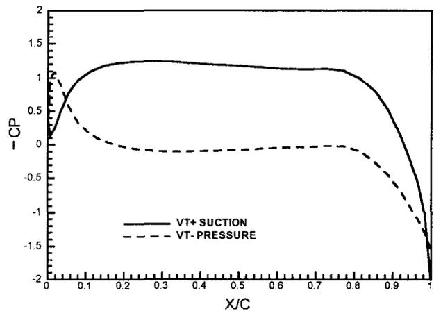
Fig. 17. Maximum and minimum blade pressure distribution,  $r/R = 0.811$ ,  $J_A = 0.876$
