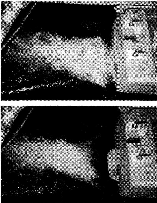
Fig. 11. Model-scale transom flow comparison, baseline (upper) and with stern flap (lower), full load, 16 knots
