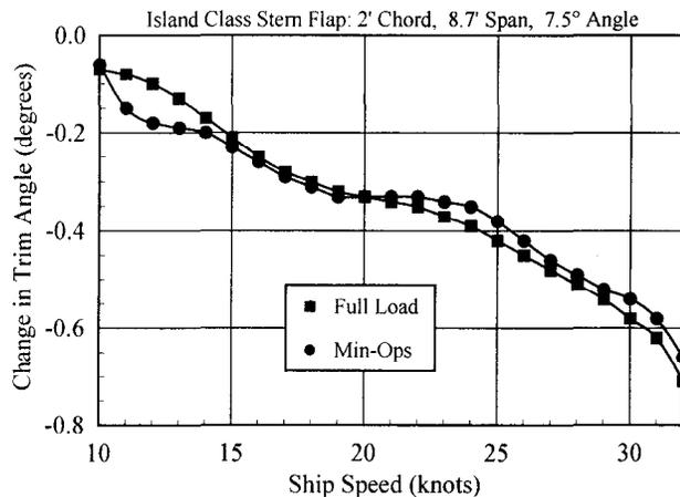
Fig. 7. Selected stern flap #6, effect on ship running trim
