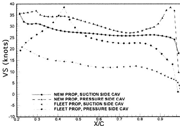
**Fig. 22.** Predicted cavitation inception speeds, at the design point, for both pressure and suction sides
