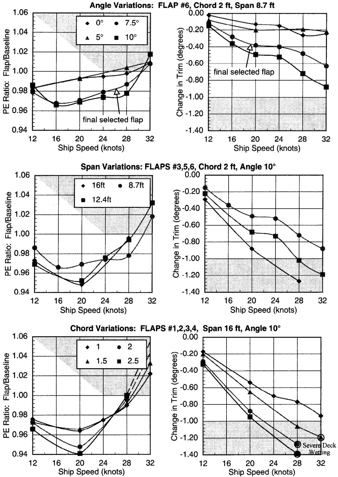
Fig. 4. Examples of results of model-scale stern flap optimization experiments (Stern flap scale effects are not included)
