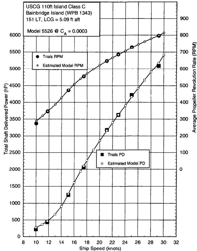
**Fig. 2.** Ship/Model comparison: *BAINBRIDGE ISLAND* (WPB 1343) versus Model 5526, 151 L. tons, correlation allowance 0.0003
