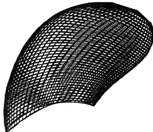
Fig. 18. Propeller blade grid distribution
