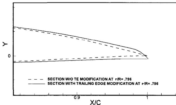
Fig. 20. Propeller blade sections, with and without trailing edge modification,  $r/R = 0.796$
