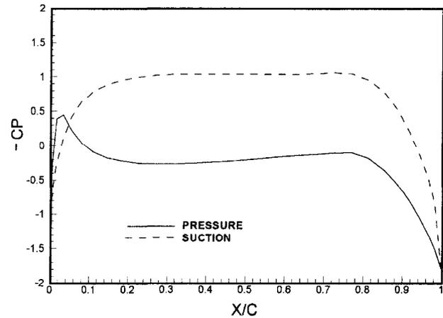
Fig. 16. Circumferential average blade pressure distribution,  $r/R = 0.811$ ,  $J_A = 0.876$
