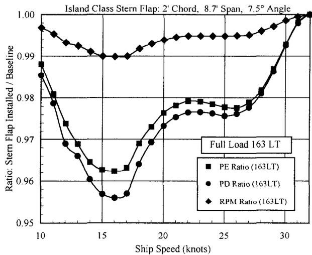
Fig. 5. Model-scale performance of selected stern flap #6, Full Load condition of 163.39 L. tons
