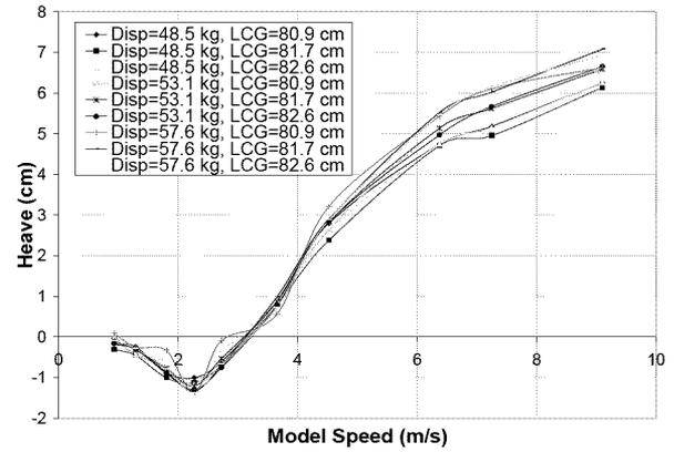
Figure 15: Heave versus speed for the free-to-sink-and-trim condition.
