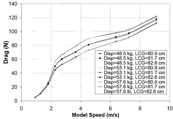
Figure 13: Drag versus speed for the free-to-sink-and-trim condition.
