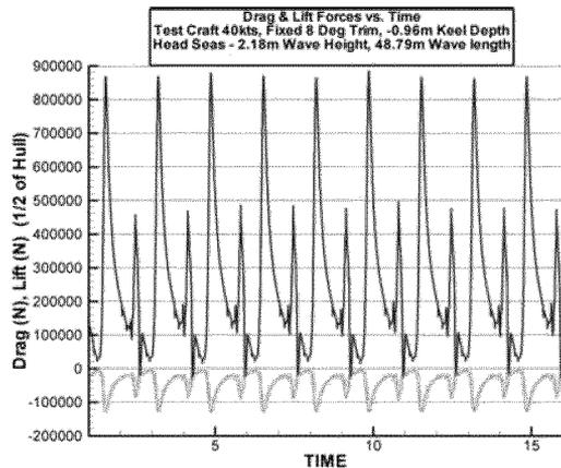
**Figure 2: Drag and lift predictions for ½ of the hull at 40 knots in head sea waves.**
