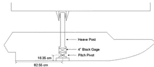
**Figure 5: Towing schematic for the free-to-sink-and-trim condition.**
