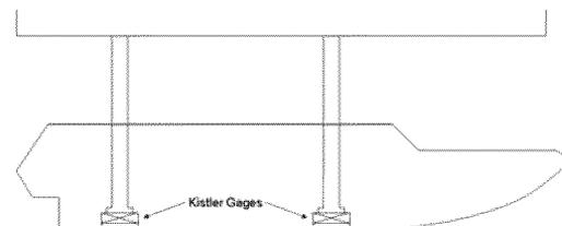
**Figure 4: Towing schematic for the fixed condition.**
