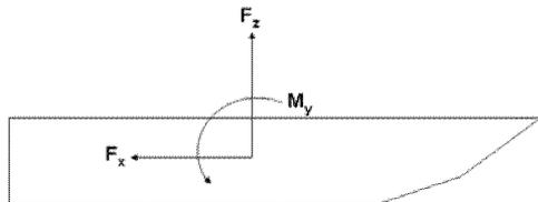
**Figure 6: Side view of the monohull showing the force orientation.**
