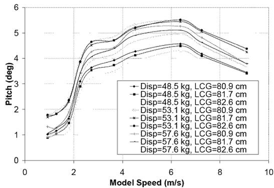
Figure 14: Pitch versus speed for the free-to-sink-and-trim condition.
