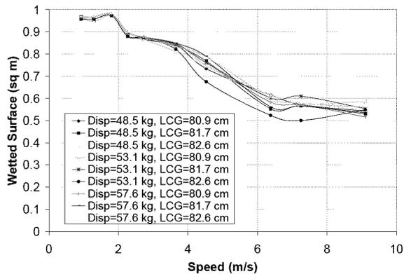
Figure 18: Wetted surface versus speed for the free-to-sink-and-trim condition.
