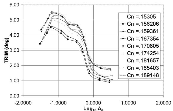
**Figure 23: Trim versus the log of Almeter Number for Model 5658.**
