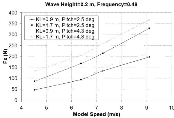
Figure 9: Average peak drag versus speed for fixed in the smaller wave condition.
