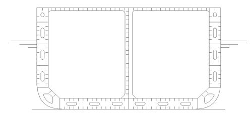
Fig. 1: Double Hull Tanker Midship Section
