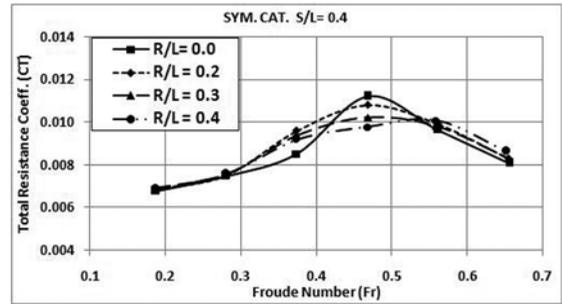
Figure 6:  $C_T$  values of staggered symmetrical catamaran,  $s/L=0.4$ .
