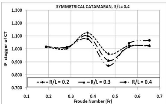
Figure 12:  $C_T$  values of  $IF_{stagger}$  symmetrical catamaran,  $s/L=0.4$ .
