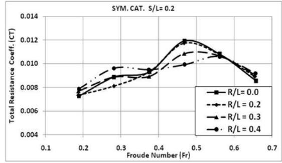
Figure 5:  $C_T$  values of staggered symmetrical catamaran,  $s/L=0.2$ .
