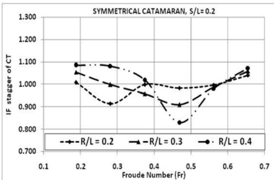
Figure 11:  $C_T$  values of  $IF_{stagger}$  symmetrical catamaran,  $s/L=0.2$ .
