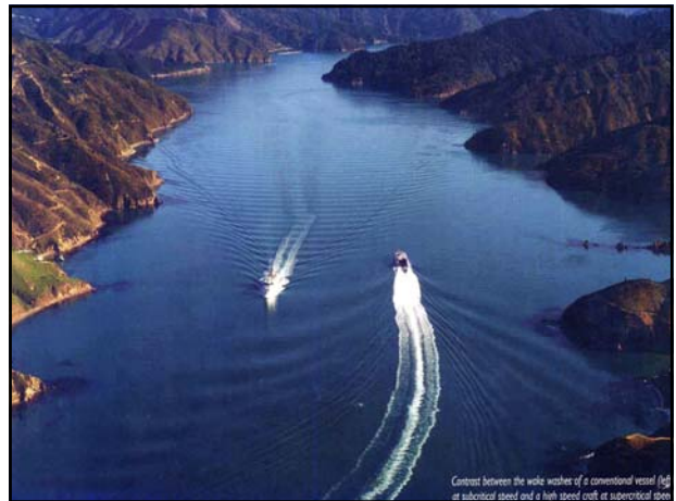
Contrast between the wave washer of a conventional vessel (fig. at subcritical speed) and a hull steered out at supercritical speed
