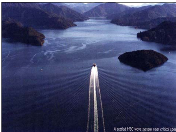
A settled HSC wave system near critical speed
