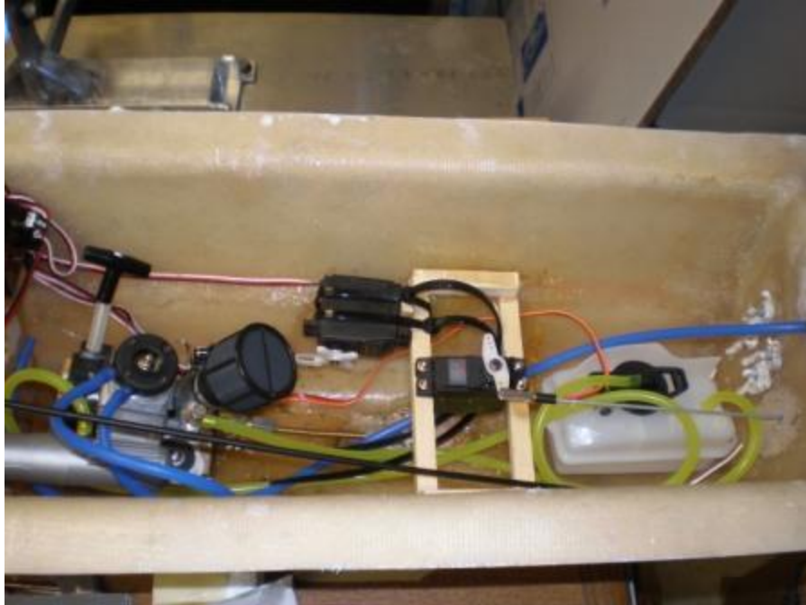
Figure 5.7.2: Complete installation of servo systems
