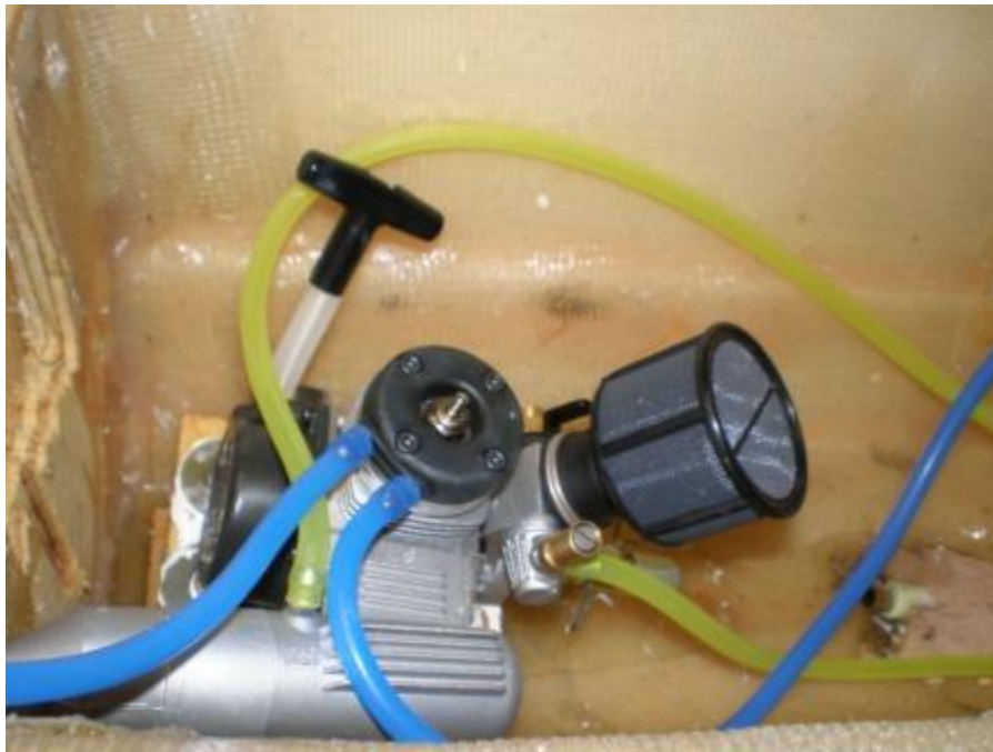
Figure 5.5.4: Engine in place on mount with color coded tubing connected
