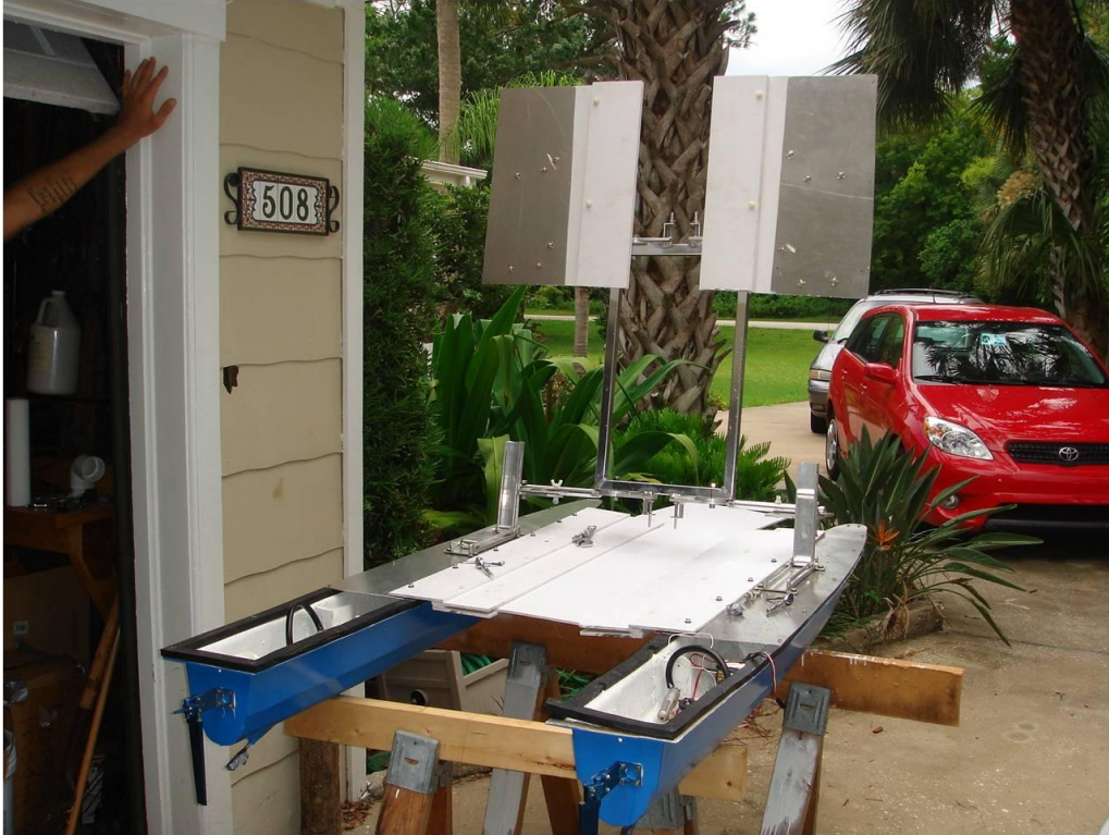
Figure 5.9.1: CODAC completely assembled with engine hatches open.
