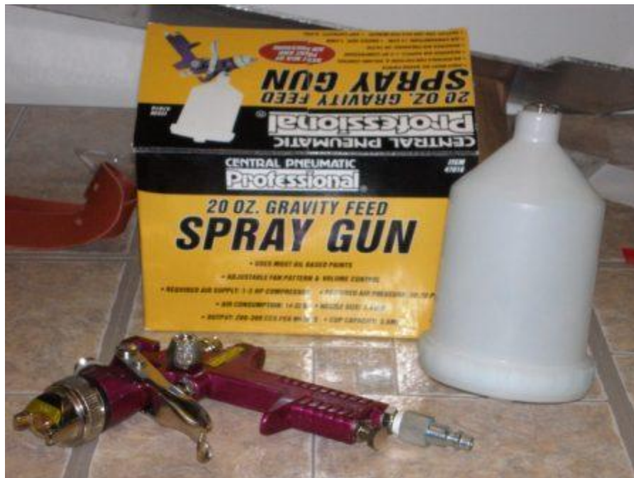
Figure 5.4.2: Gravity feed spray gun used for enamel coat.
