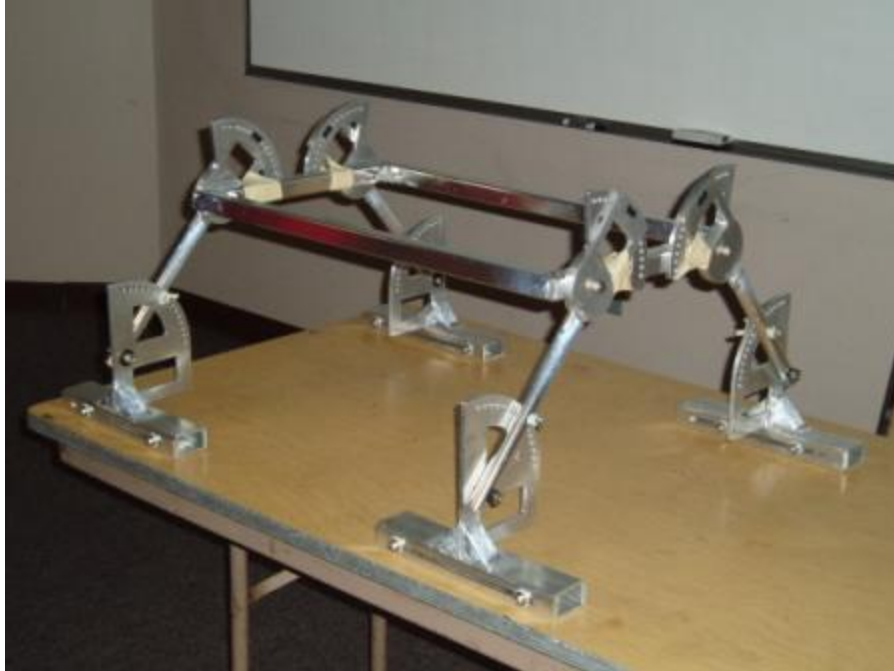
Figure 5.1.4: Complete spacing structure ready for assembly onto hulls
