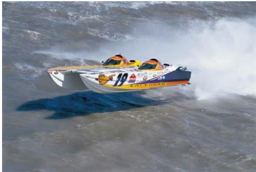
Figure 2.3.2: An example of the grounding effect in a catamaran (MARINE PERFORMANCE/RACE ENGINES, 2007)
