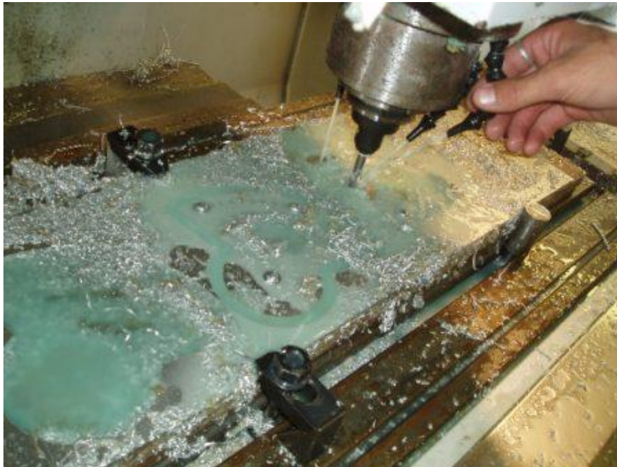
Figure 5.1.1: CNC milling of structural cams
