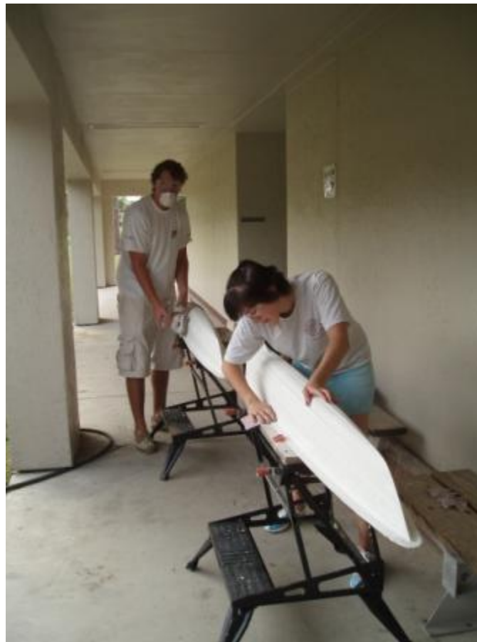
Figure 5.4.1: Sanding of hulls in preparation of painting
