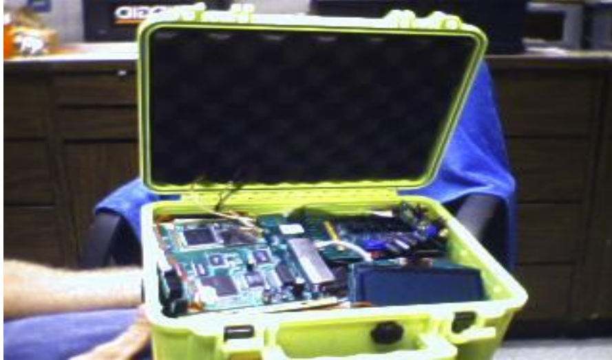
Figure 6.2.1: Electronics package for data acquisition in new waterproof case
