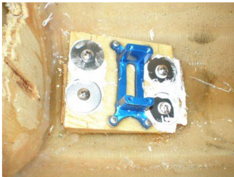
Figure 5.5.3: Full engine mount installed in hull
