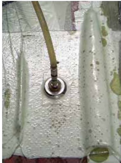
Figure B-3: Model plug for centre hull and outrigger under vacuum
