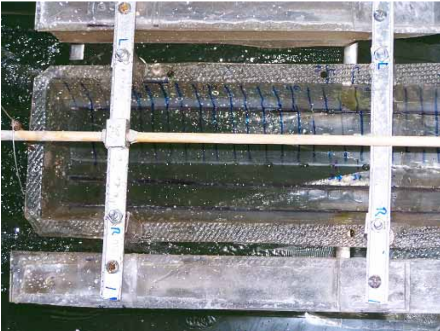
Figure 6.4: Model test photo for determining wetted surface area
