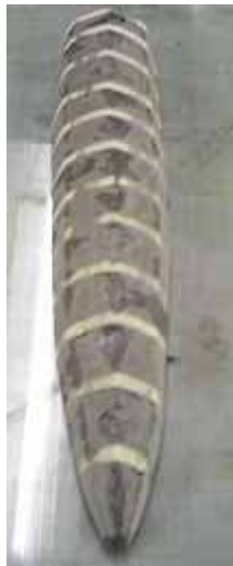
Figure B-2: Faired hull, ready for glass coating
