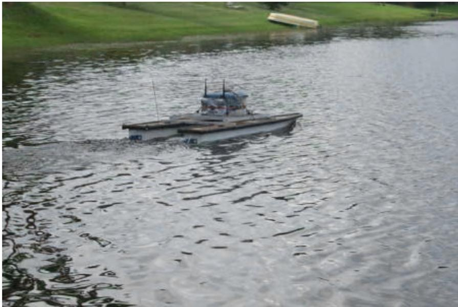
Figure 6.1.2: Displacement hull being tested in calm water
