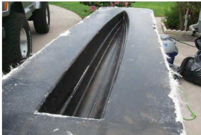
*Figure 4.2.12: Mold after foam removal.*
