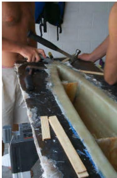
*Figure 4.2.16: Attempting to release the first prototype hull from the mold.*
