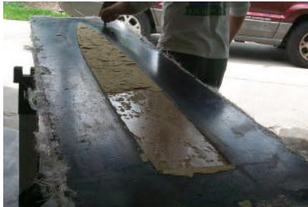
*Figure 4.2.10: Foam portion of plug inside mold after delaminating from base*
