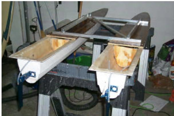
*Figure 4.2.25: Forward portion of the deck mounted to the hulls*
