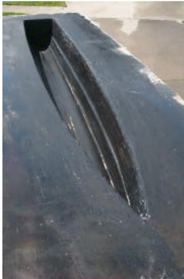
*Figure 4.2.13: Completed mold after bondo and sanding work*
