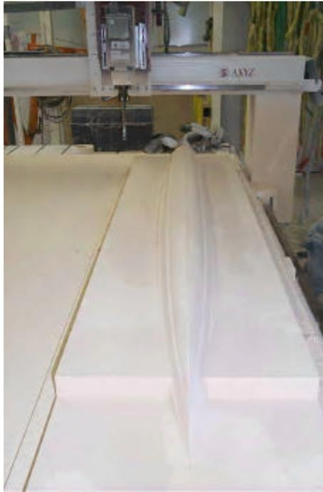
*Figure 4.2.2: The foam plug in between cuts on the CNC machine.*
