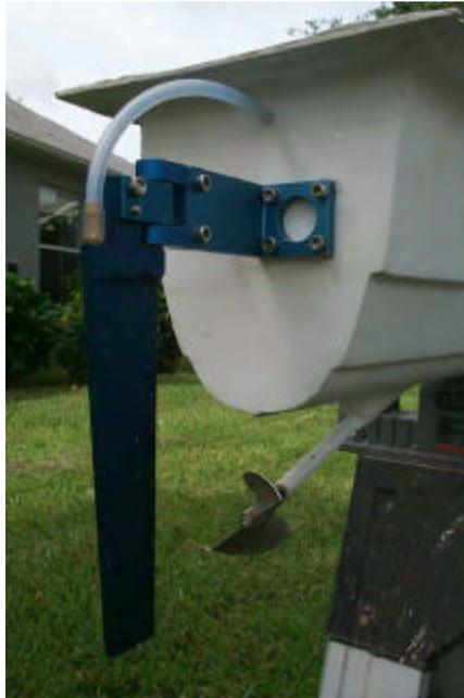
*Figure 5.2.2: Rudder (with attached cooling system) and propeller used for steering*
