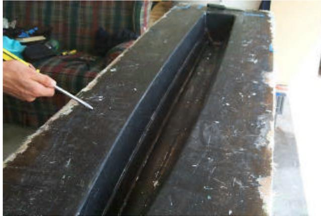
*Figure 4.2.18: Mold after removal of the first prototype hull.*
