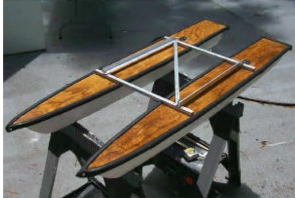
*Figure 4.2.26: Prototype after rub rails were cut and added around the lips of the hulls.*
