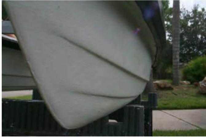
Figure 4.2.29: Detailed view of chine running down the port side hull
