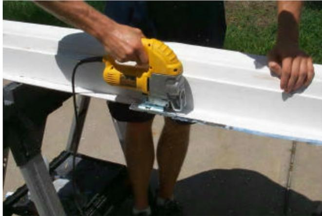
*Figure 4.2.21: Using a jig saw to cut the edges of the prototype hull*
