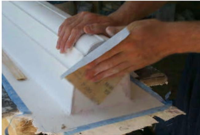
*Figure 4.2.20: Sanding the stern portion of the second prototype hull*
