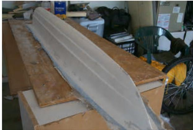
*Figure 4.2.17: First prototype hull after removal from the mold.*
