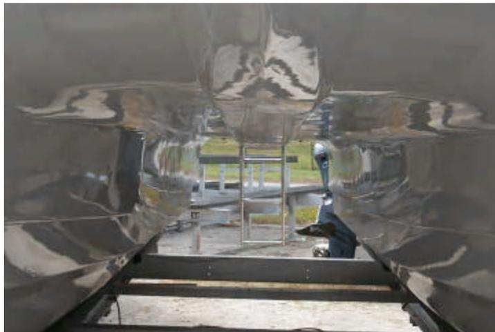
*Figure 7.3.1: The tunnel of a Glacier Bay Canyon Runner 2665*
