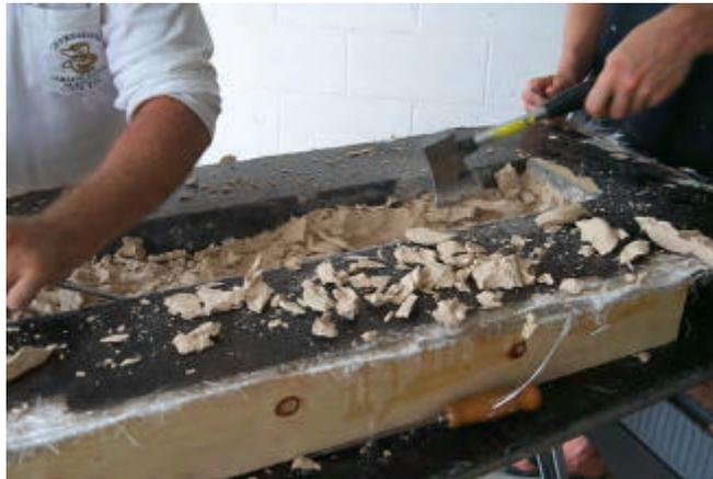
*Figure 4.2.11: Foam being chiseled out of mold*
