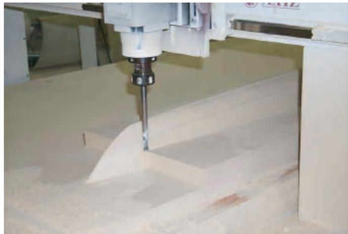
*Figure 4.2.1: The CNC mill cutting the foam for the plug.*
