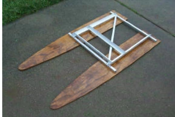
*Figure 4.2.24: Finalized connection system bolted to the decking*
