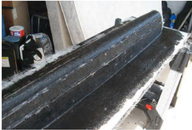
*Figure 4.2.6: Layer one of fiberglass over plug to create the mold.*
