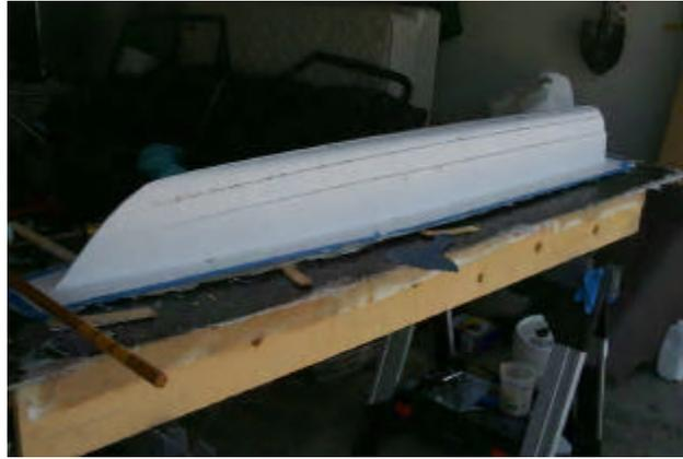
*Figure 4.2.19: Second prototype hull after removal from the mold.*
