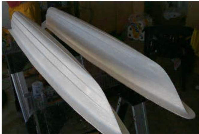
*Figure 4.2.22: Hulls after the application of a layer of gelcoat*
