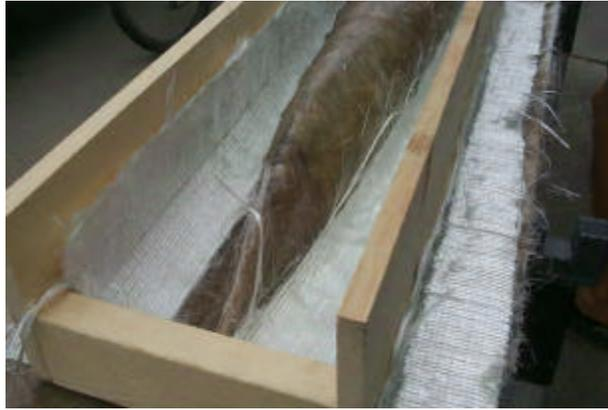
*Figure 4.2.9: The wood being set around the mold to act as a base*
