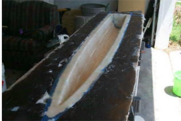
*Figure 4.2.14: First layer of fiberglass curing in the mold*
