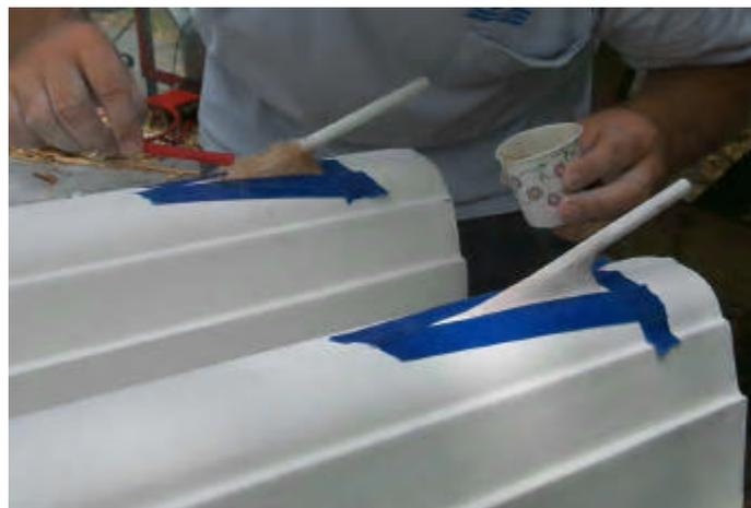
*Figure 4.2.27: Adding chopped strand mat over drive shafts to seal them*
