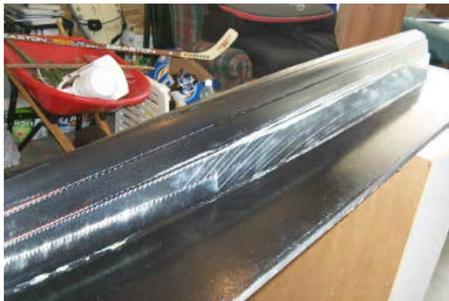
*Figure 4.2.5: Plug after application of the paste wax, leaving a smooth shiny surface.*
