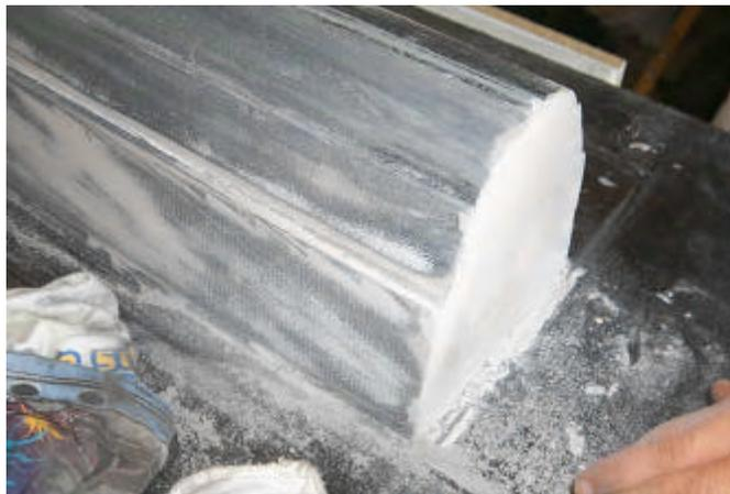
*Figure 4.2.3: The stern portion of the plug following bondo application and sanding.*
