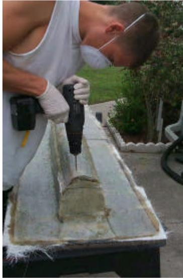
*Figure 4.2.7: Drilling holes in the mold over the air pockets*
