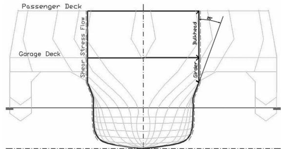
Figure 10.- Pentamaran hull forms adapted to create an “Internal Monohull”
