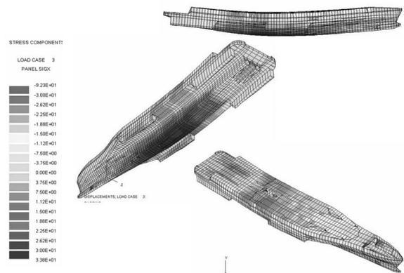
Figure 18.- Longitudinal stresses (MPa) for the sagging condition. Deformed x100
