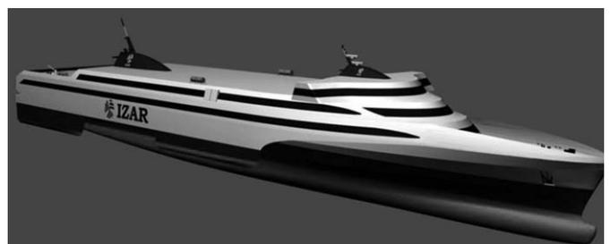
Another effect associated to the non-standard hull configuration has been detected. While the forebody is nearly a monohull, the aft body is more like a trimaran. This means that, during a complete hogging-sagging cycle, the loads are flowing in the structure in a quite different manner, depending on the number of sponsons submerged at each time step, leading to peculiar shear lag effects.
