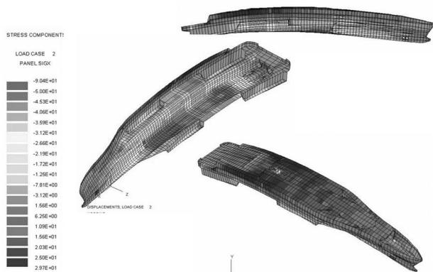
Figure 16.- Longitudinal Stresses (MPa) for the Hogging Condition. Deformed x 100
