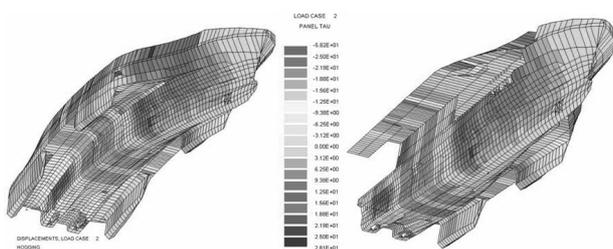
Figure 19.- Shear stress (MPa) for Hogging Condition outer (Def x100) and inner views
