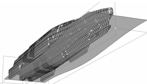
Figure 17.- Sagging wave in the FE model
