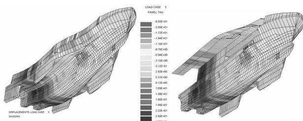
Figure 20.- Shear stress (MPa) for Sagging Condition outer (Def x100) and inner views
