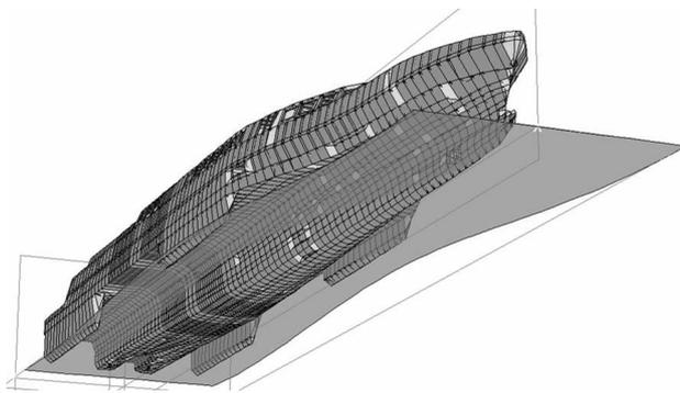
Figure 15.- Hogging Wave in the FE Model
