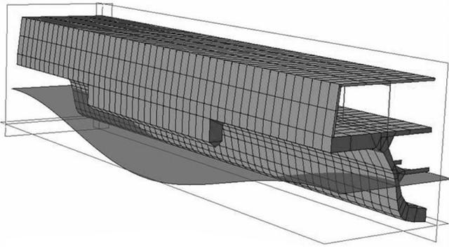
Figure 5.- Midship Section Extruded Model
