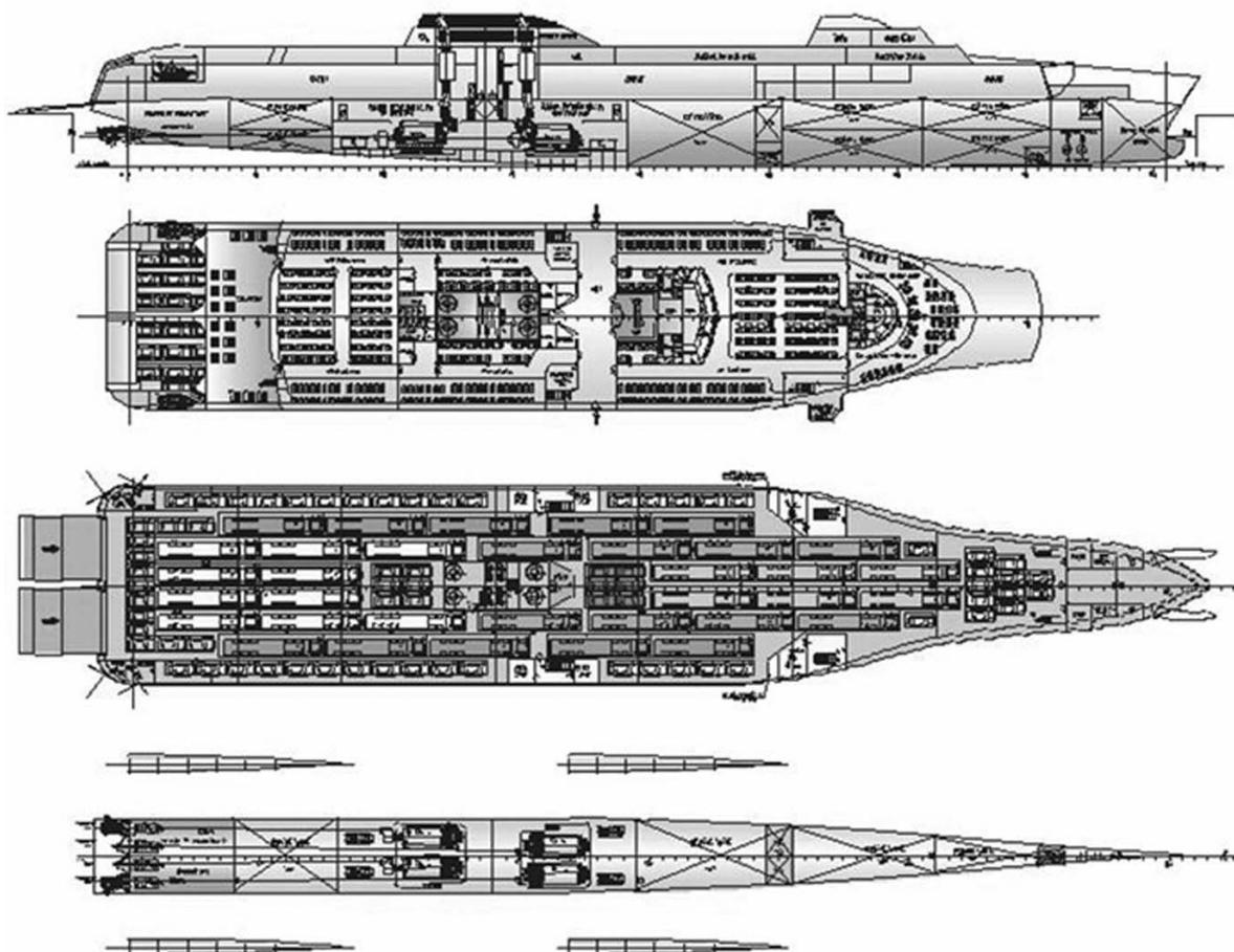
Figure 4: General Arrangement of the Basic Pentamaran
