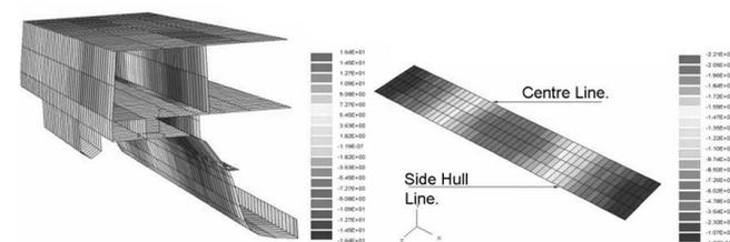
Figure 9.- Configuration with Longitudinal Bulkheads
